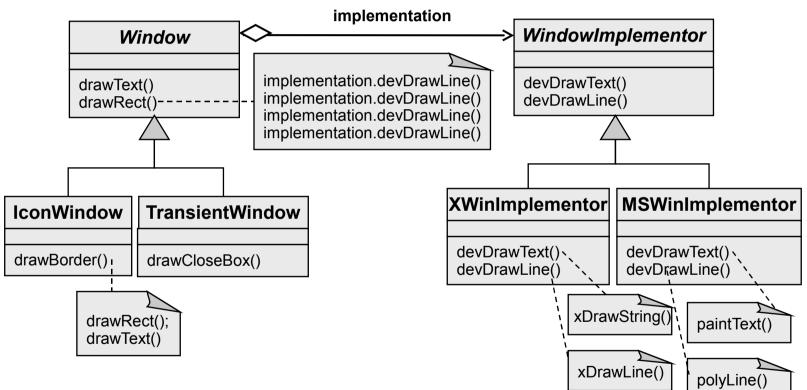
The **Abstraction classes** implement the methods of different window types in using the methods, made available by the **Implementation classes**
