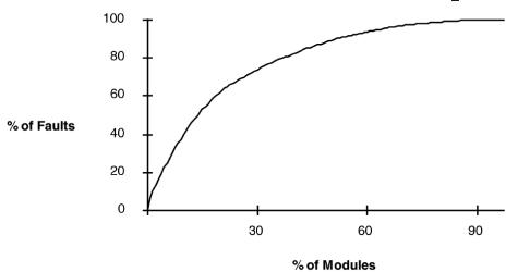
The diagram shows % of modules versus % of faults for a release n
